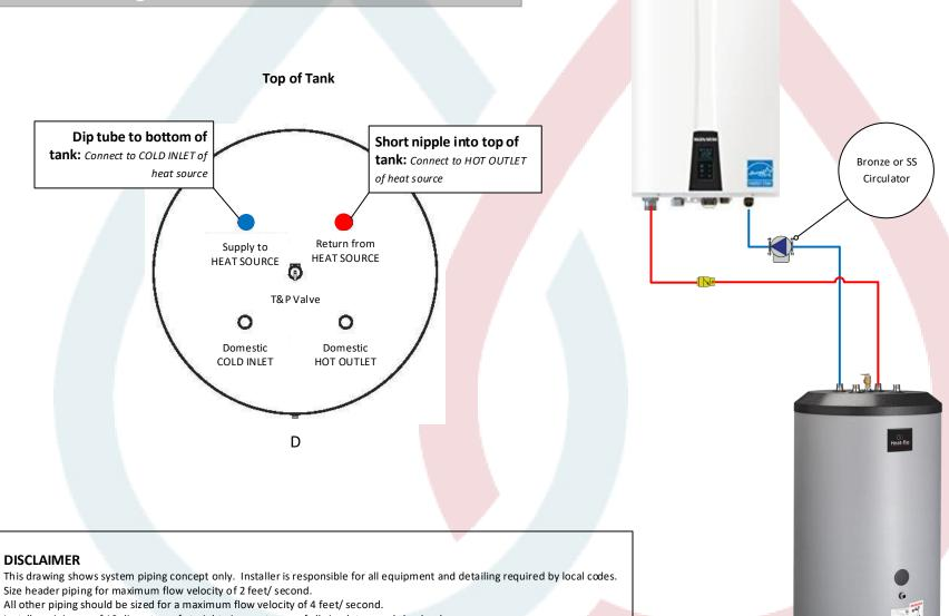
Install a minimum of 12 diameters of straight pipe upstream of all circulators and check valves.
